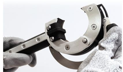
9. Fit the trimmer blade in place by aligning the guides with the groove
