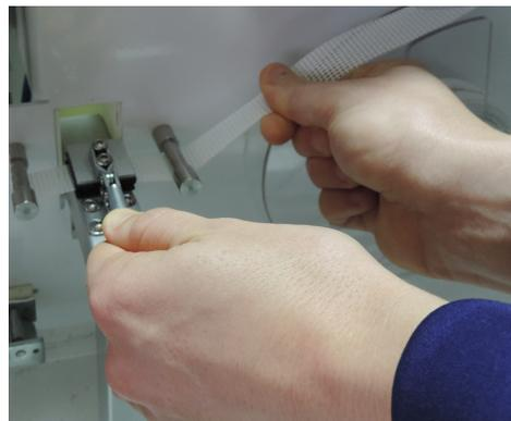
21. Clamp the media in place using the lever attached near the clamping jaws of the media clamp
