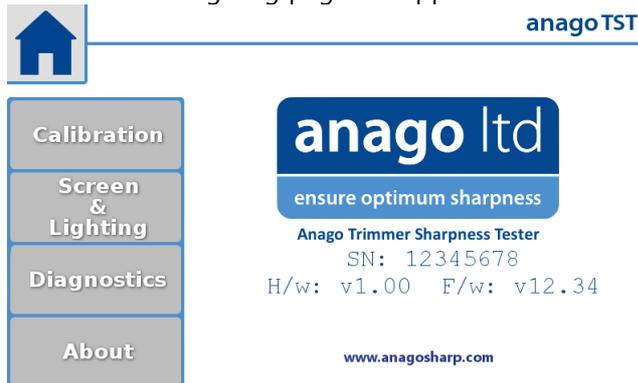
The firmware version is stated after "F/w:". In the example shown, the firmware version is 12.34.
